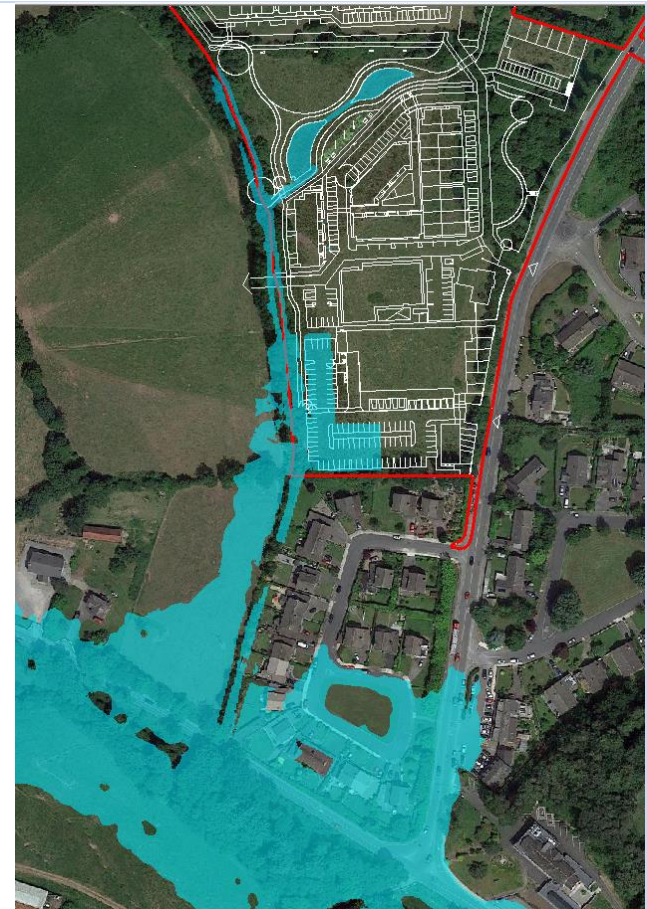
Fig 3.6c - Developed terrain, stream flow = 0.1%AEPCC (2.2m 3 /s), river = 1%AEPCC (44m 3 /s)
