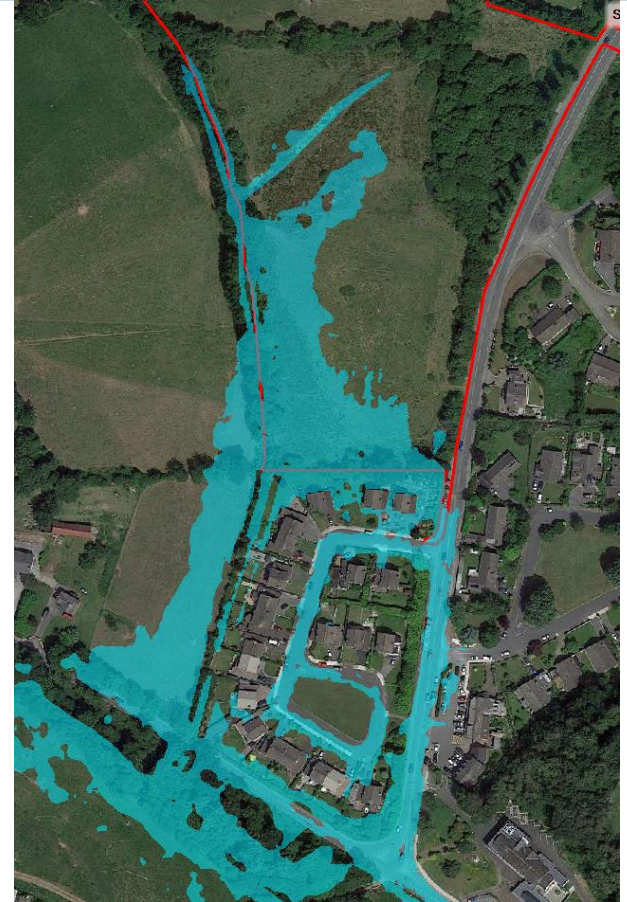
Fig 3.2c - Existing terrain, stream = 0.1%AEPCC (2.2m 3 /s), river = 10m 3 /s
