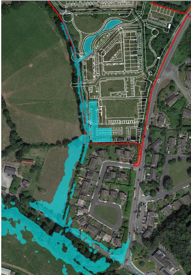
Fig 3.5a - Developed terrain, stream = 1%AEP (1.4m 3 /s), River = 10m 3 /s
