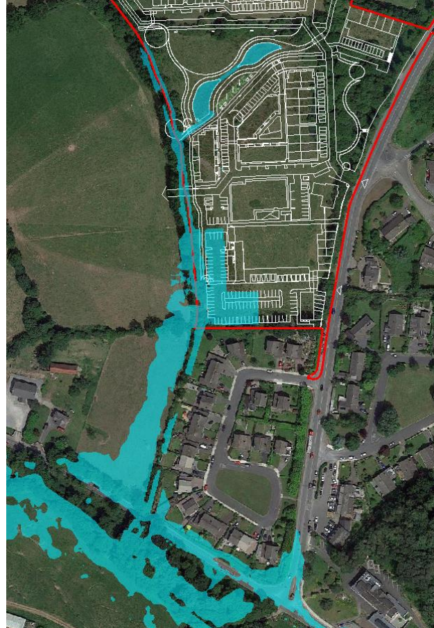
Fig 3.5b - Developed terrain, stream = 1%AEPCC (1.7m 3 /s), river = 10m 3 /s
