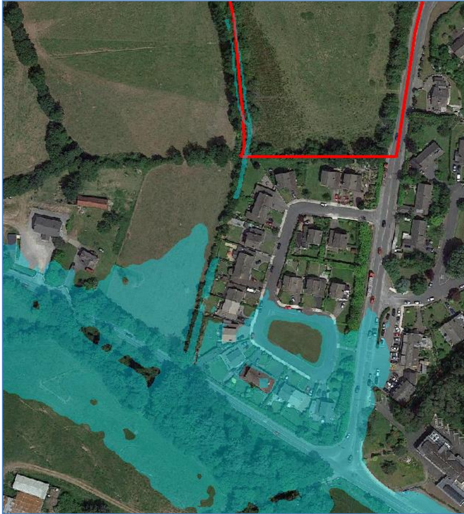
Figure 3.1-Extent of inundation arising from 1% AEPCC peak flow in river and a nominal flow in the western stream ( 0.2\text{m}^3/\text{s} )
