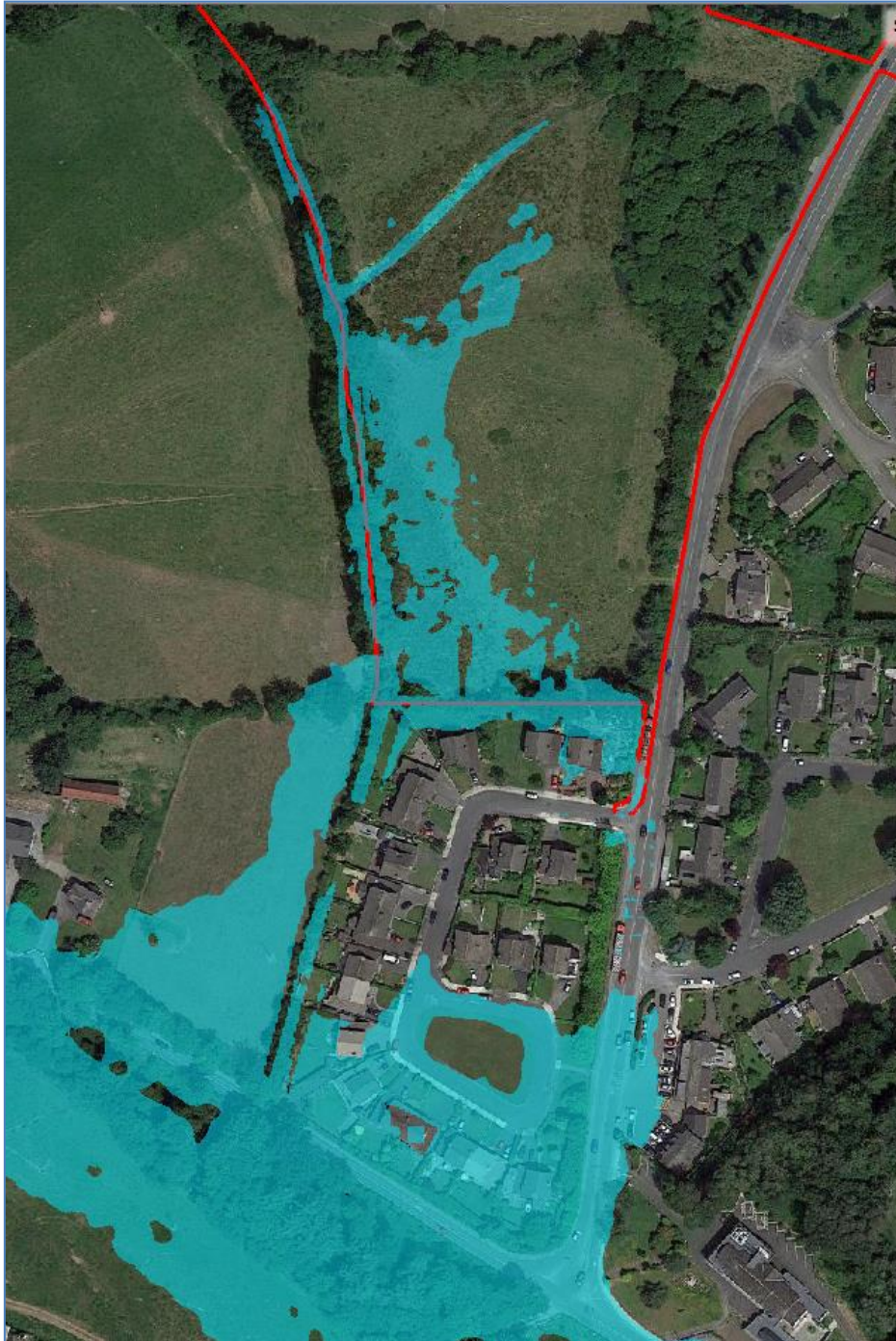
Figure 3.15 -Flood Zone A areas as defined by the 1%AEP flood event in the stream
