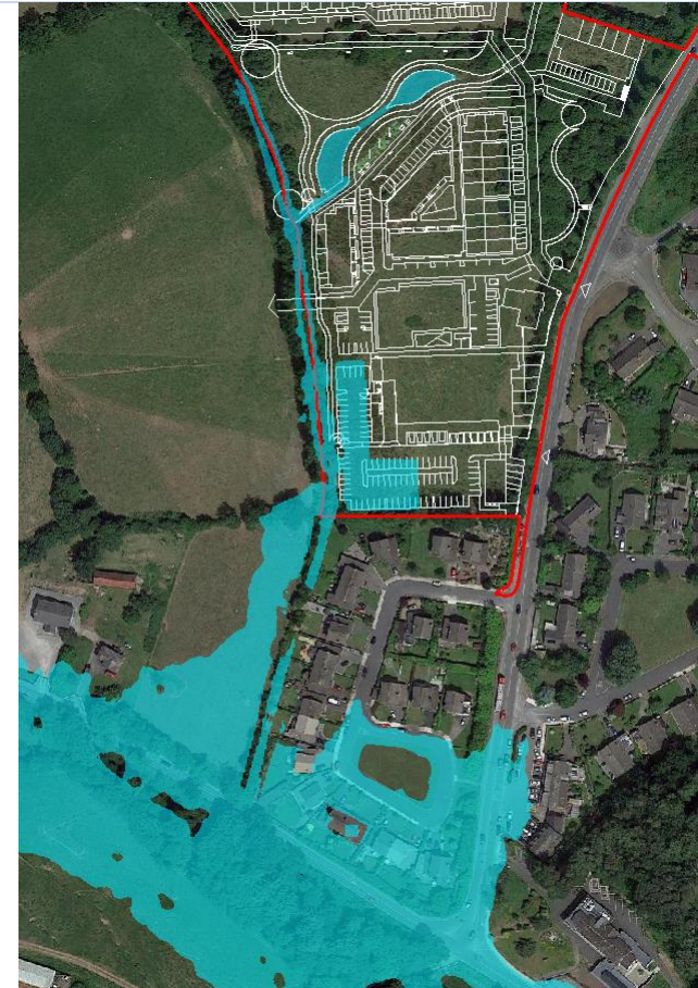
Fig 3.6a - Developed terrain, stream = 1%AEP (1.4m 3 /s), river = 1%AEPCC (44m 3 /s)
