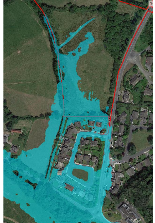
Fig 3.3c - Existing terrain, stream = 0.1%AEPCC (2.2m 3 /s), river = 1%AEPCC (44m 3 /s)
