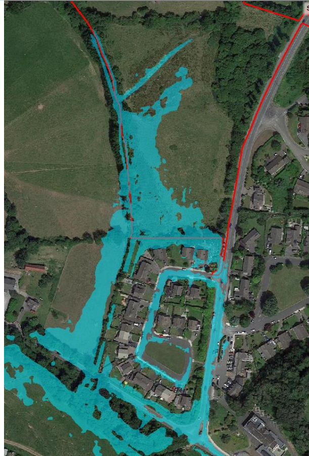
Fig 3.2b - Existing terrain, stream = 1%AEPCC (1.7m 3 /s), river = 10m 3 /s
